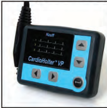
Figure 1 CardioHolter Digital Holter ECG Monitor
